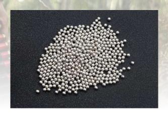
Agescan's bismuth shot products were proudly manufactured under ASTM B774-00 and ISO9001 standards. With a compound of 94% bismuth and 6% tin, we achieve a density range of 9.58-9.67 g/cm3, ultra-high purity, small grain size and outstanding pellet integrity.
